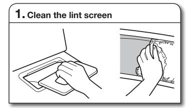
Clean the lint screen before each load. Pull the lint screen out of its holder. Roll lint off the screen with your fingers. Do not rinse or wash screen to remove lint. Push the lint screen firmly back into place.
